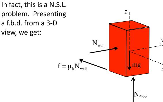
The floor's *normal force* does nothing as the floor is frictionless, but the wall's *normal force* is important because it is not only provides the centripetal force needed to motivate the body along a curved path, it is also the quantity that determines the accelerating *frictional force* in the *negative x-direction*.
